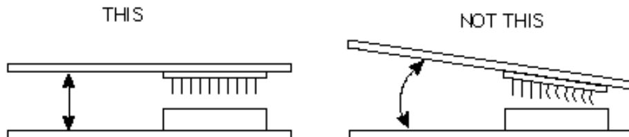
Figure 1-48. Separating CPU and Master I/O
